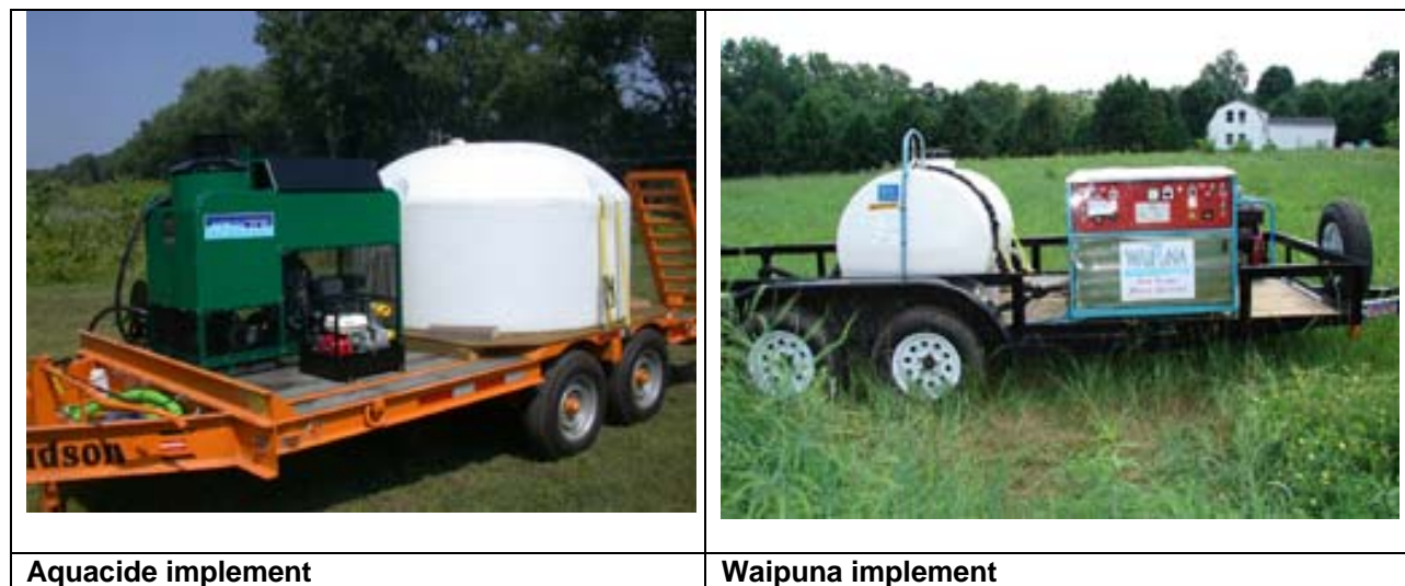
Figure 4.28. Steam application equipment used in research.
